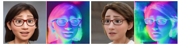
Figure 9: Limitations. If the input subject wears eyeglasses, strong discontinuity in normal values near the glasses may hinder reliable surface normal integration.
